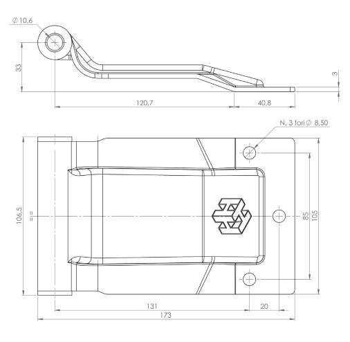
The new external hinge MH 100 was born from the market's need for a product with a new design and geometric features, completely different from traditional hinges. Consequently, Pastore & Lombardi has developed a new hinge, preserving the mechanical properties of their hinge type MEDIUM, currently on sales, and achieving a weight reduction of about 35%
